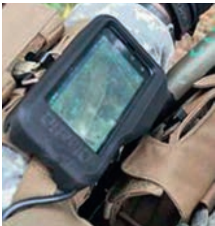
MAINGATE man-wearable radio met Next Generation Mobile Ad hoc Networking Waveform
