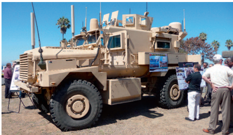
UHF SOTM Antenna Installed on Bushmaster (on top, front) en de SOTM X/Ka band antenne van L3 (on top rear)
